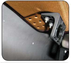
7 Secure Angled Seat Bracket (F) to hull by threading a 10-32 X 1 Truss Bolt (G) through a 10-32 Neo Bond Washer (H), secure with a 10-32 Nylon Locknut (I) Repeat to other bolt and other side.
