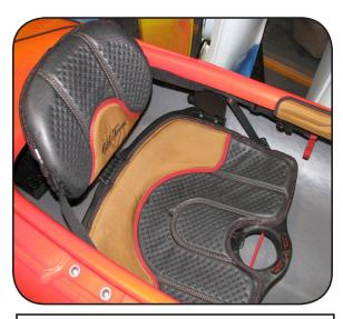
1. Remove old seat with a phillips head screwdriver. You may need to rotate the seat 90 degrees in order to remove it from the cockpit.
