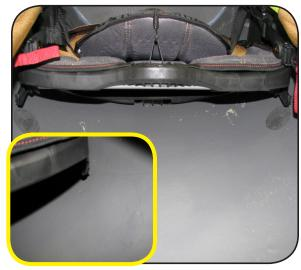
9. Lower seat pan to lowest position and lightly press down to leave marks on inside hull. Flame marks and center a Bumper Pad (J) on each mark left or hull. lower seat base. Adjust seat back straps and enjoy your new seat!
