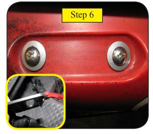
6. Each seat back strap has a plastic plate with tabs (See Fig). These plates must be slid between seat bracket and hull with tab facing down to hold bracket in place (See Fig). CAUTION: Straps must not be twisted. Insert 2" X 14 Truss Screws (D) through 7/8 SS Sealing Washer (E), thread through kayak, Seat bracket. Repeat to other bolt and other side.
