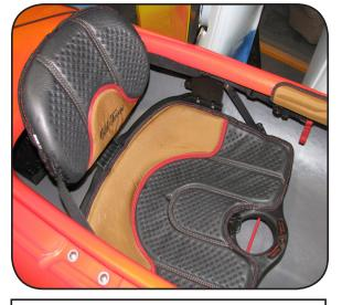
3. Insert the ACSII Seat Assembly (A) into the cockpit and check tower to floor fit. The towers should be tight and the seat base tight to the floor of the kayak. If seat is tight from towers to floor, tighten tower bolts and proceed to step six.
