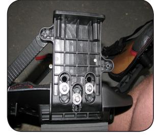
4. If towers are short remove the three bolts and adjust the height to best fit. Reinstall bolts, washers, and tighten.
