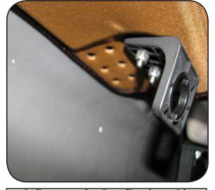
2. Remove the Seat Bracket with a phillips head driver and 3/8ths wrench.
